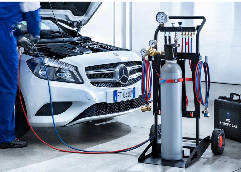
Meets Daimler AG's requirements for gas detectors because Forming Gas is a non-polluting and readily available gas mixture that consists of 95% nitrogen and 5% hydrogen.
