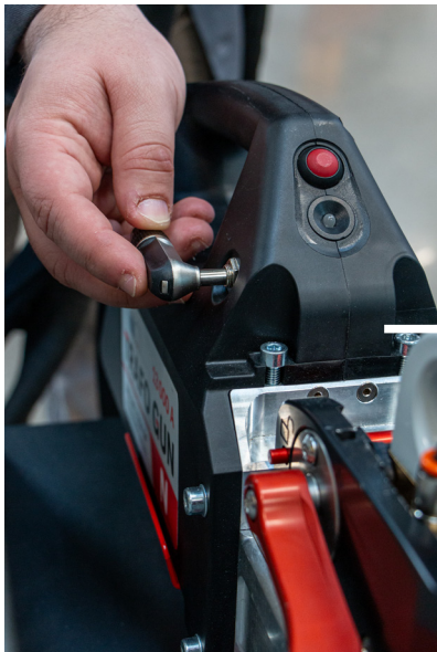
Connecting the control cable from the gun to the clamp
