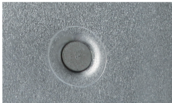
RESULT OF THE INSTALLATION OF SELF-PIERCING RIVET
