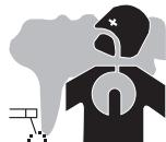
The fumes, gases and dusts emitted by welding are hazardous to health. Sufficient ventilation must be provided, and an air supply is sometimes necessary. A fresh-air mask can be a solution if ventilation is inadequate. Check that the extraction system is effective by checking it against safety standards.
