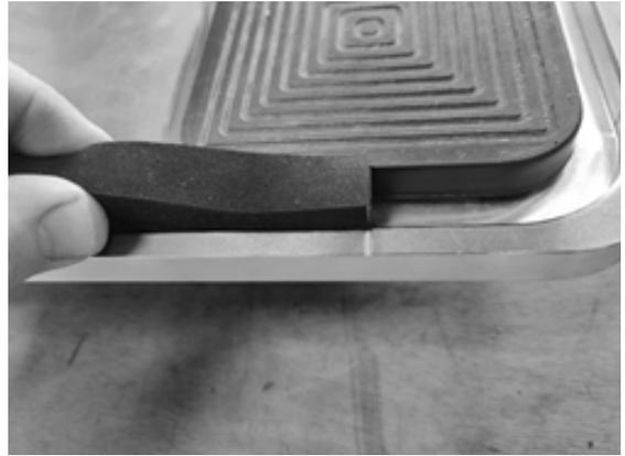
Pinch the gasket into place in the groove.
