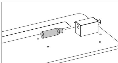
Screw the silencer onto the Venturi block by hand
